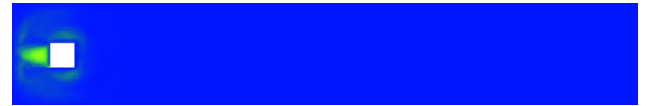
Figure 4: The dual velocity on the finest mesh for goal functional M1 (drag).
