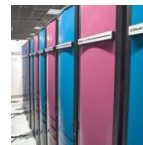
Louhi: Cray XT4/XT5 with 2.3 GHz 4-core AMD Opteron. All-in-all 9424 cores and Peak power of 86.7 Ttlops.
